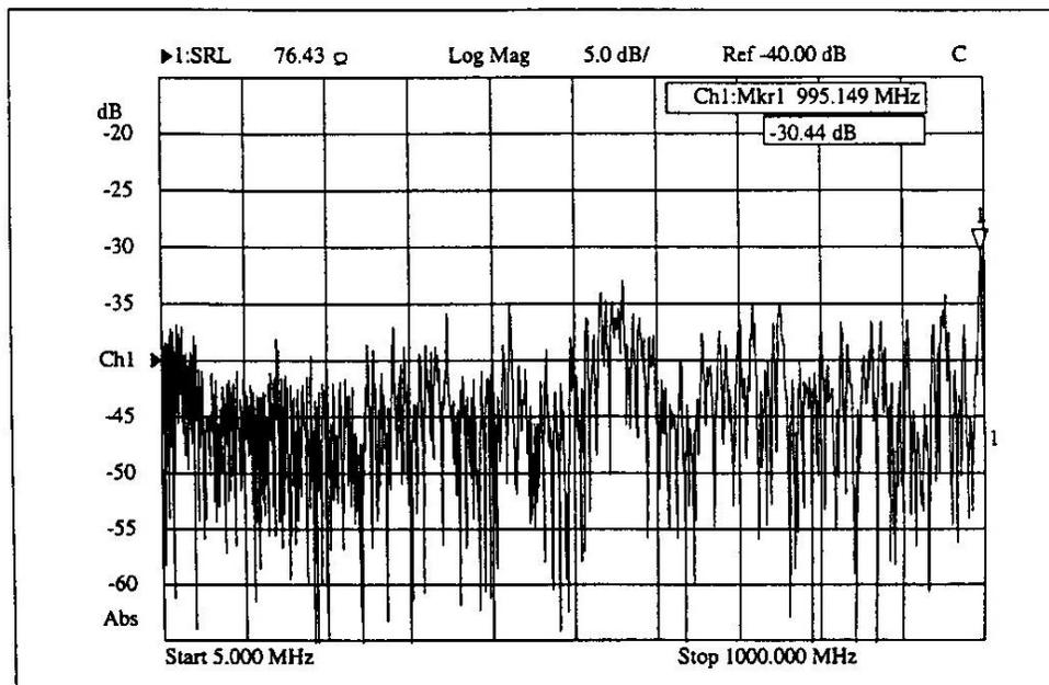
Figure 2 – Example Display of Structural Return Loss – Fixed Bridge Method
