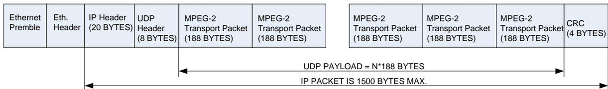
Figure 6–1 - MPEG-2 Transport Stream over UDP/IP
