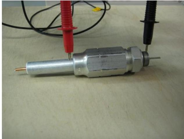
**Figure 3 - Test Leads Attach Points (2)**
