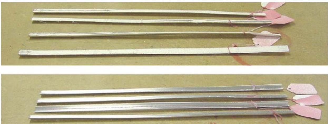
**Figure 3 - Samples cut in half and with dielectric removed**
