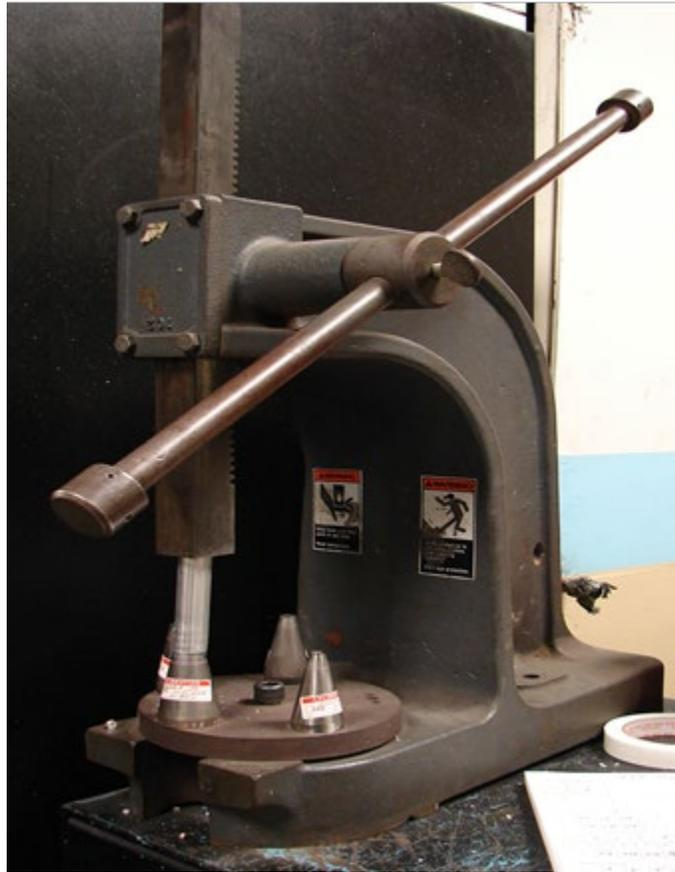
Figure 6 - Mechanical Arbor Press
