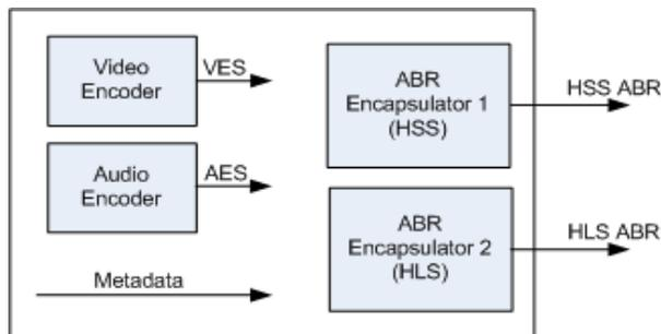
**Figure 8 - Unified Transcoder/Encapsulator**
