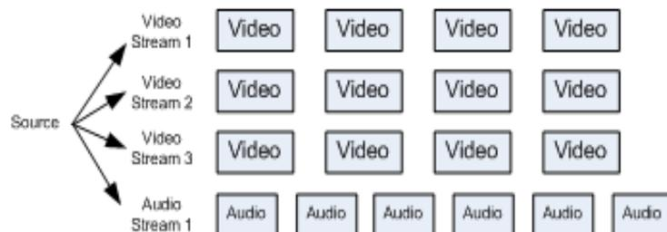
**Figure 2 - ABR with audio durations different than video**
