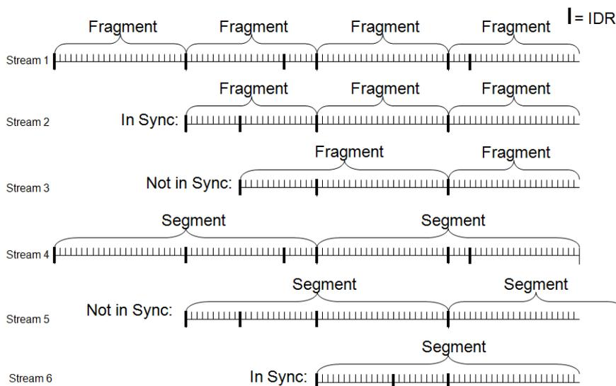
**Figure 7 - Fragment and Segment Sync/Alignment**
