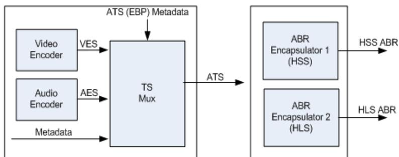
**Figure 9 - Separate Transcoder/Encapsulator with ATS in between**
