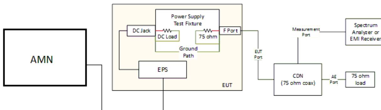
Figure 2 - Setup for Standalone Power Supplies tested with the Power Supply Test Fixture
