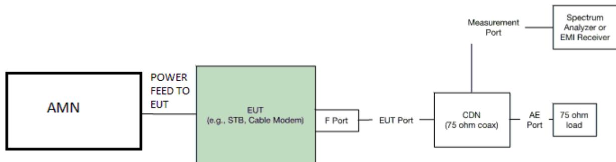
Figure 3 - Setup for Devices with Integrated Power Supplies
