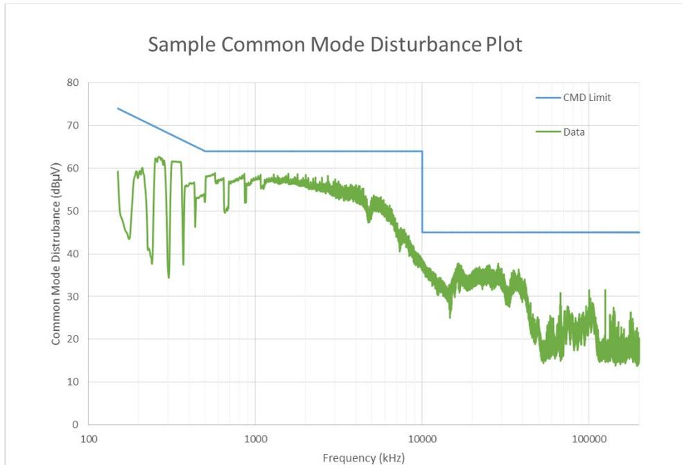
**Figure 4 - Sample Common Mode Disturbance Measurement**
