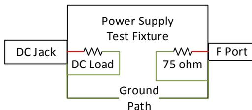
**Figure 1 - Power Supply Test Fixture**
