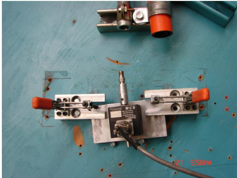
End of sample opposite to the drive portion of the flex tester shall be supported so that the end remains centered during the flexure cycle. This may be accomplished on of several ways: spindle supported in bearing assembly or encoder, or a low-coefficient of friction plug with ability to connect to the CUT during flexure.
