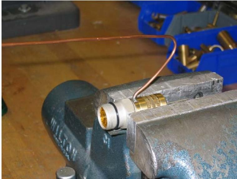
**Figure 2d - Connector body with pointer and retaining nut in vice**
