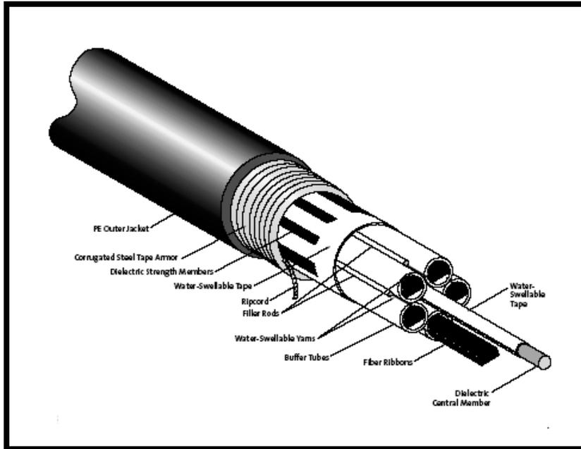
**Figure 4 – Stranded Loose Tube Cable (Ribbonized Fibers)**
