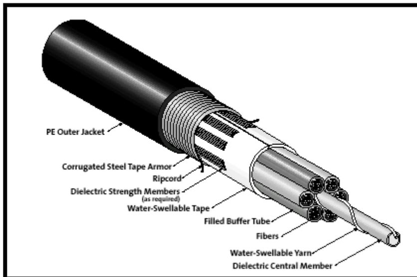
**Figure 3 – Stranded Loose Tube Cable (Bundled Fibers)**
