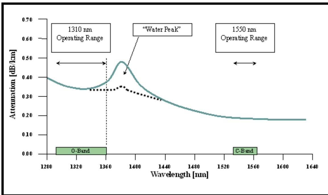
**Figure 2 – Spectral Attenuation Curve for Optical Fiber**
