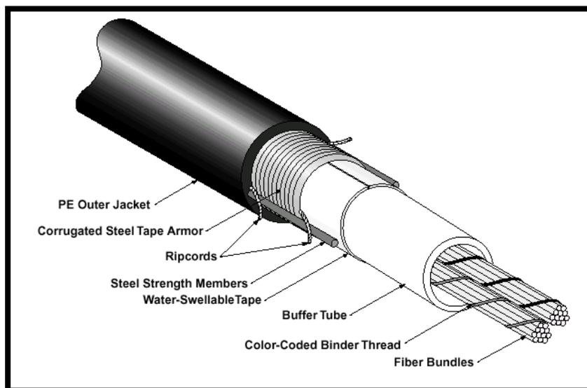
**Figure 5 – Central Tube Cable (Bundled Fibers)**
