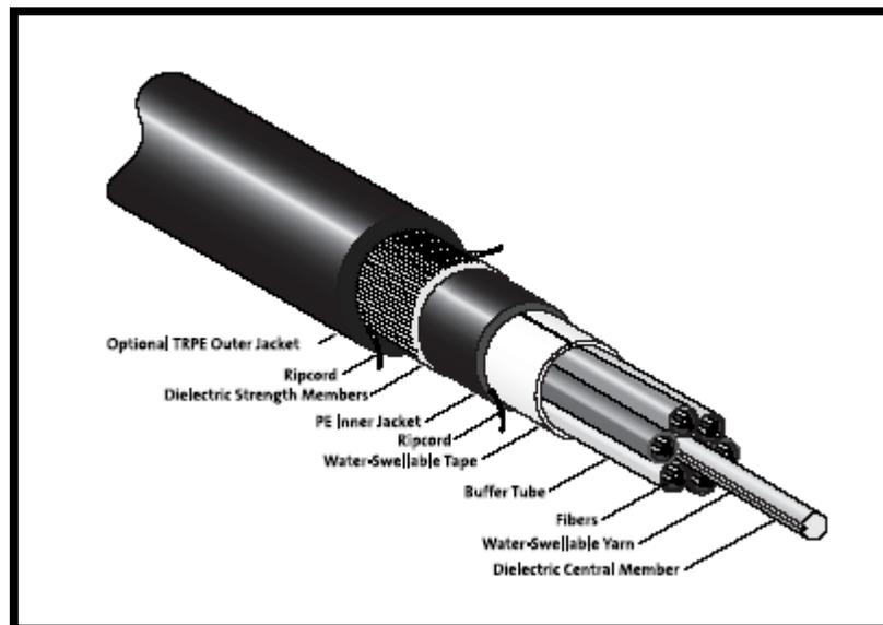
**Figure 7 – All Dielectric Self Supporting (ADSS) Cable Design**
