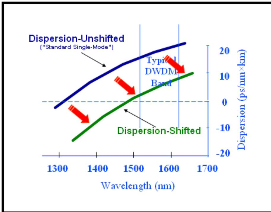
**Figure 1 – Chromatic Dispersion in Optical Fiber**
